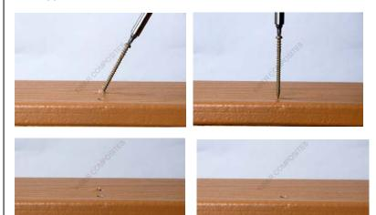
Result of angling the fastener vs. driving straight. SplitStop Titan III fastener shown.
